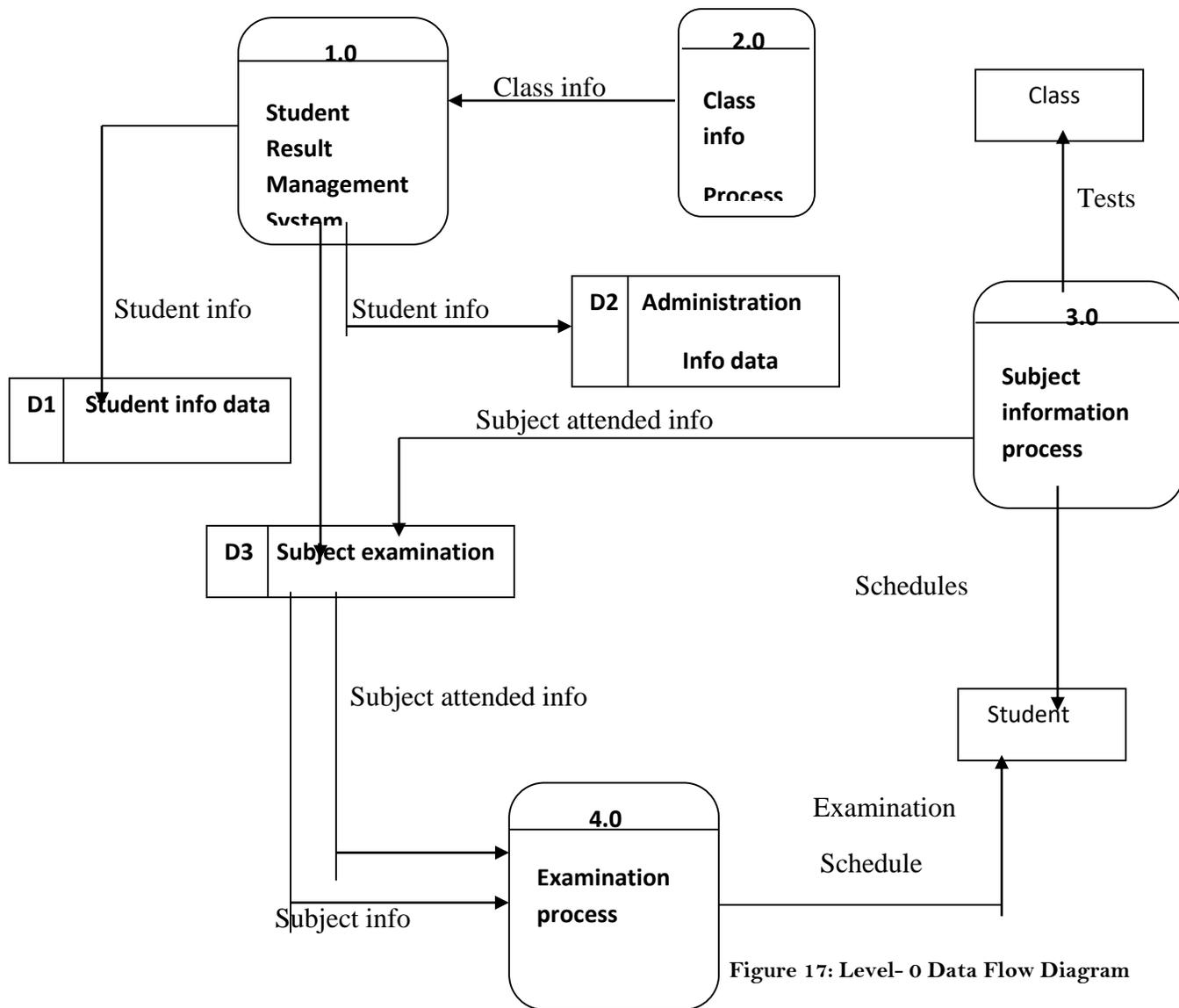
Figure 17: Level- 0 Data Flow Diagram
