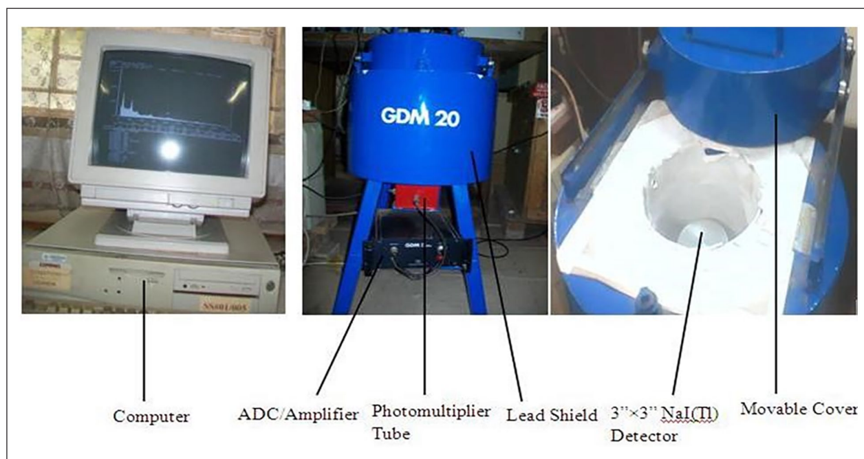
Figure 2. GDM 20 NaI(Tl) gamma ray detector.
