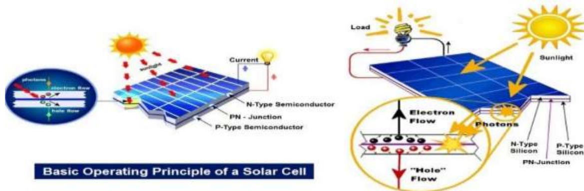
**Figure 3: Solar cell, PV solar panel, and PV panel array [11]**
