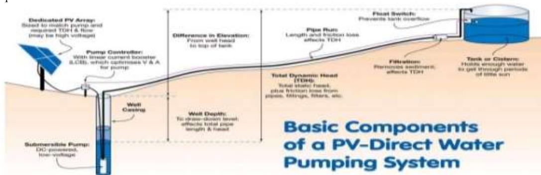
Figure 4: Schematic diagram of solar powered water pump system [23]
