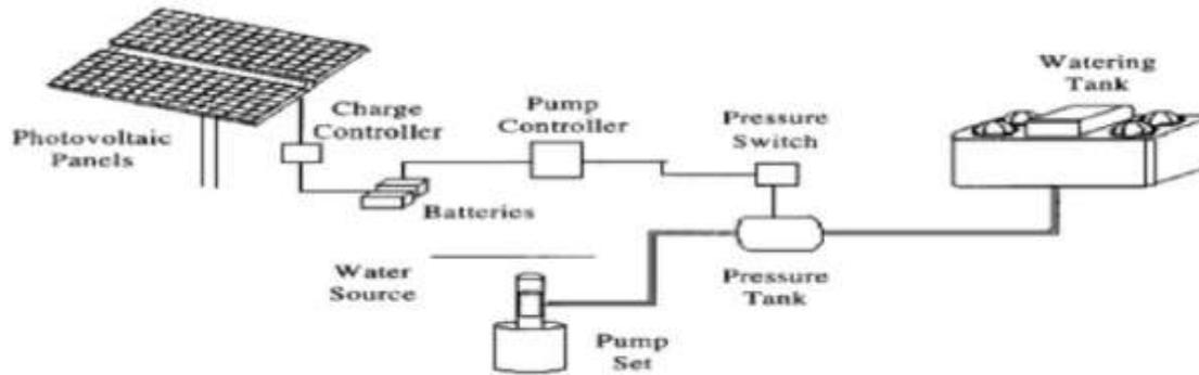
Figure 5: Battery-Coupled Solar Water Pumping System [23]
