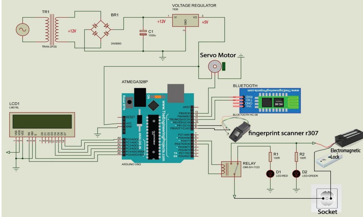
**Figure 7: Circuit Diagram of AHSDCS**
