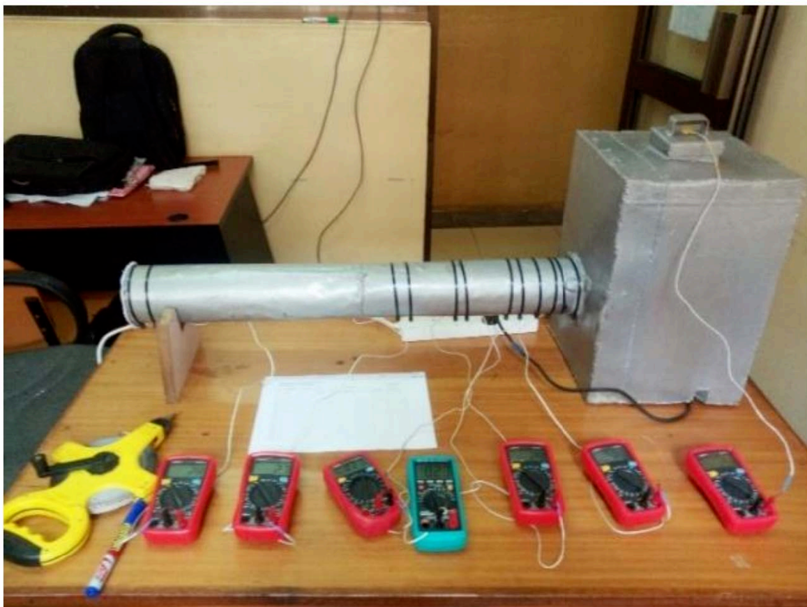
Fig. 1: Insulation testing rig with a projected cylindrical test surface.
