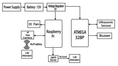
Fig2. The block diagram of the system
