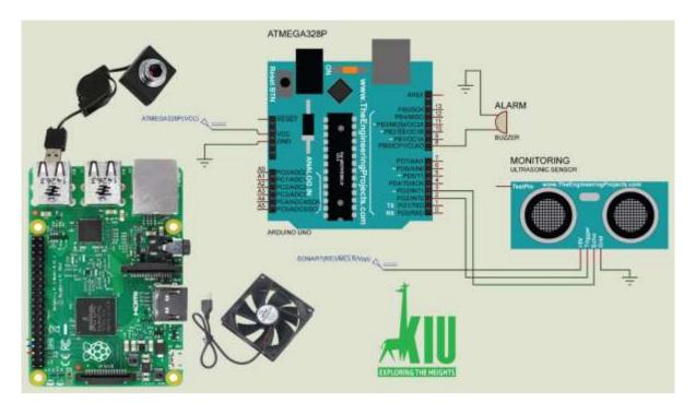
Fig3. The circuit diagram of the system
