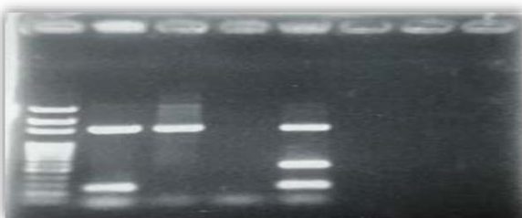
Figure 3. Agarose gel electrophoresis 1% of the multiplex PCR amplification products of the "mecA" and "nuc" genes, from S8 to S10 of the strains tested (SmartLader 200bp, Eurogentec).
