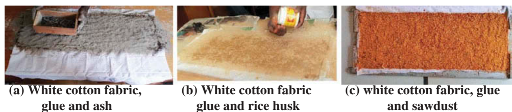
Figure 2. Development of composite insulating materials.
