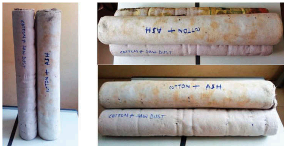
Figure 3. Developed composite insulating materials.
